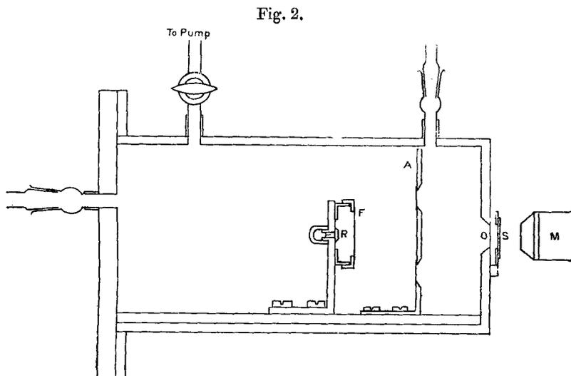
The sheet of paraffin was held on a diaphragm placed at A, equidistant from the source R and the ZnS screen. The opening O was covered with aluminium foil of 3.7 cm. air-equivalent, and absorbing screens of aluminium could be inserted between the opening and the ZnS screen. These screens were necessary to prevent scattered  $\alpha$  particles from hitting the ZnS screen, and were also used in measuring the range of the H particles.
