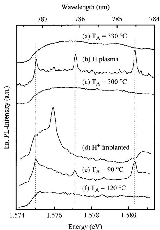
FIG. 2. PL spectra of a CdTe crystal that was (a) pre-annealed, (b) treated in a hydrogen plasma at 160 °C, and (c) subsequently annealed. For comparison, PL spectra of a CdTe crystal are shown that was (d) H<sup>+</sup> implanted at 50 °C, and (e) and (f) subsequently annealed at different temperatures.
