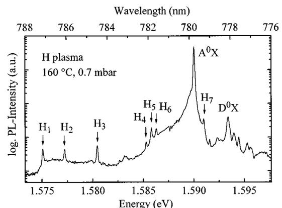
FIG. 1. PL spectrum of a CdTe crystal treated in a hydrogen plasma for 1 h.
